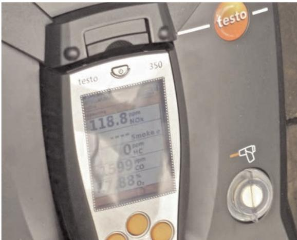
....as can be seen by the pictures taken by myself, shown here, taken of the readings on the Testo professional gas analyser and the exhaust particulates test card. I can therefore confirm that this was what I witnessed. The SulNOx fuel appeared to have produced an enormous improvement.
