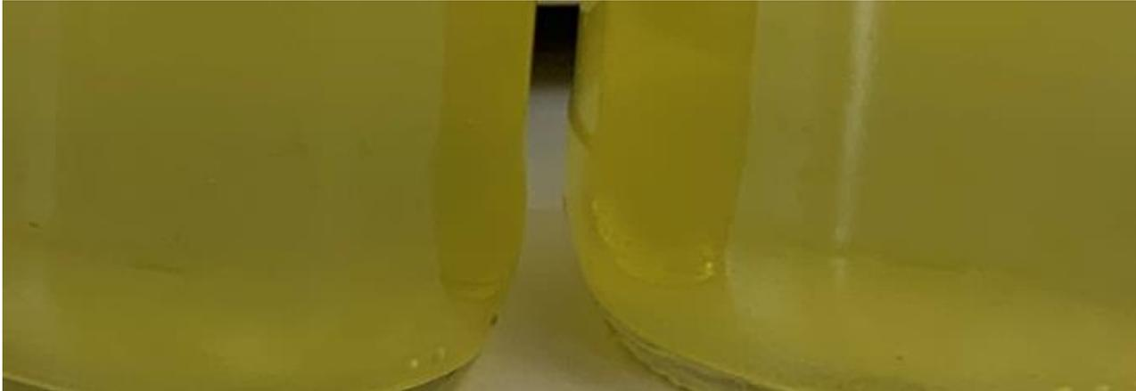
(Figure 1.4. Formulations 4 & 5. Emulsified diesel with no precipitation)
